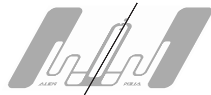
Angular Sensitivity Inlay is rotated in the x, y, plane about the z axis
